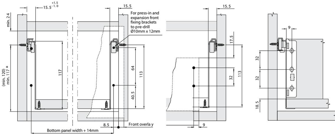
( ) Inner Drawer \* Add 8mm when used with 201.000 Drawer Front Locking Piece.
